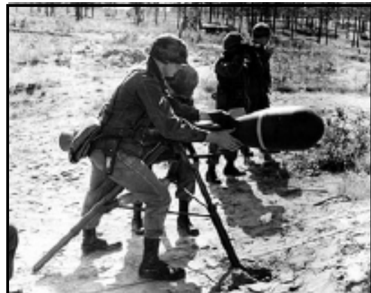
W-54 missile crew setting up 120mm version of the recoilless rifle for field test exercise.
