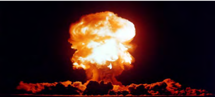
SNAPPER "DOG" ( 05-01-52 ) WAS A 19 KILOTON ( FINAL ) "PROOF" TEST OF THE "TX-7" ( MK-7 ) TACTICAL NUCLEAR BOMB ASSEMBLY DESIGNED TO QUALIFY THE USEFULNESS OF DEUTERIUM ( GAS ) FOR BOOSTING AGENT PURPOSES.
