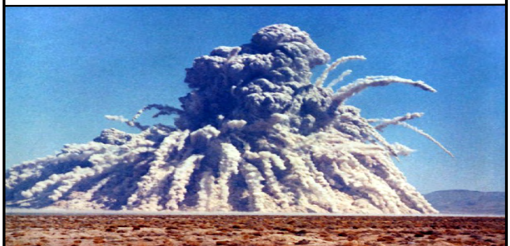
" SEDAN " was, a 104 Kiloton ( -650 ft. ) sub-surface test of a "W-56" Submarine Launched Ballistic Missile ( SLBM ) Warhead. The test was conducted at the Nevada Test Site ( NTS ) and lifted 12 million tons of rock and alluvial soil to an altitude of several thousand feet. It also dispersed 880,000 Curies of Radioiodine ( I-131 ) into the atmosphere, causing extreme health issues, including cancers and premature death to civilians who lived "downwind" of the test site.
