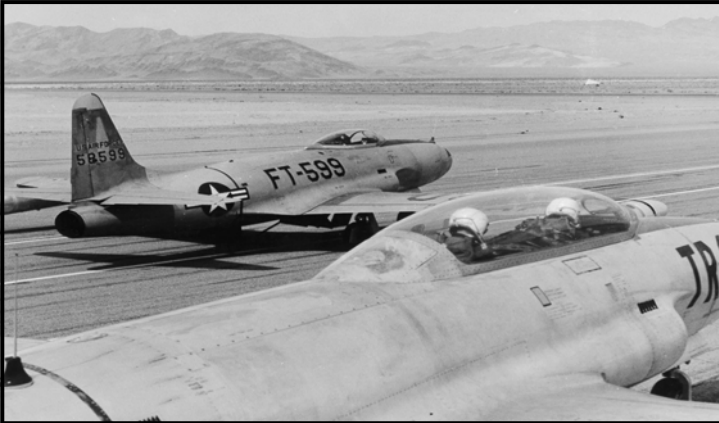
A QF-80 ( TOP ) IS ROLLING OUT FOR TAKEOFF WHILE BEING ( REMOTE ) CONTROLLED BY THE BACK-SEAT OFFICER IN THE SECOND AIRCRAFT. ....
