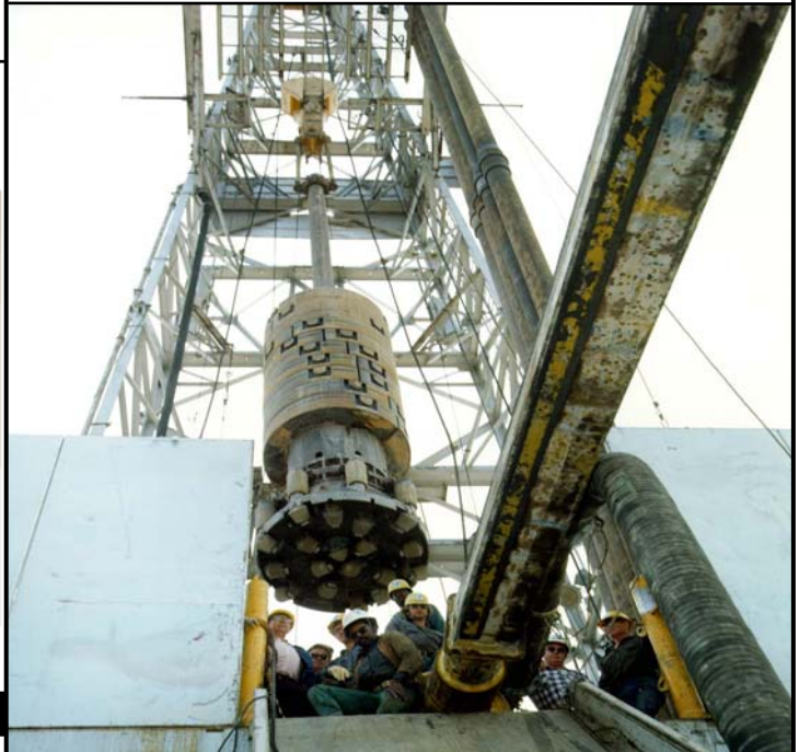
THE RIG FLOOR CREW PREPARES TO DRILL THE SHOT SHAFT FOR THE (1.2 MEGATON) "MILROW" TEST
