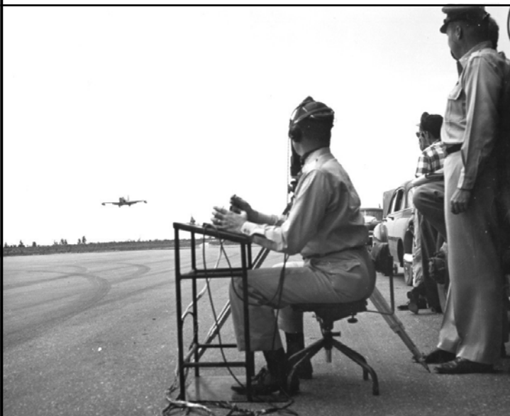
A GROUND CONTROLLER BRINGS A QF-80 IN FOR A LANDING AT INDIAN SPRINGS AFB, AFTER A CLOUD SAMPLING MISSION OVER THE NEVADA TEST SITE. ....
