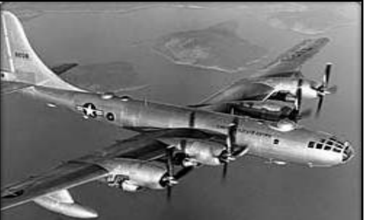
THE B-50 "BUTTER-CUP" ( A B-29 FITTED WITH LARGER ENGINES TO CARRY HEAVIER LOADS AND INSTRUMENTATION ) WAS THE DELIVERY PLATFORM FOR THE "RANGER" & "TUMBLER-SNAPPER" NUCLEAR WEAPON TEST BOMBS OVER THE NEVADA TEST SITE. . .
