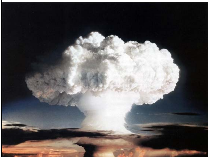
The IVY "Mike" test ( 10-31-52 ) was the first detonation of a "true" Hydrogen-Bomb device, producing a total yield of 10.4 Megatons of destructive force at Enewetak Atoll. This device weighted 82 tons, and eventually would be re-designed and up-graded to be delivered over a target from an airborne platform. The first such delivery was during the 1956 "Redwing" Series, when the "Cherokee" bomb was air-dropped ( parachute-retarded ) from a B-36-H "Peacemaker" ( high altitude ) Strategic Bomber. . . . .
