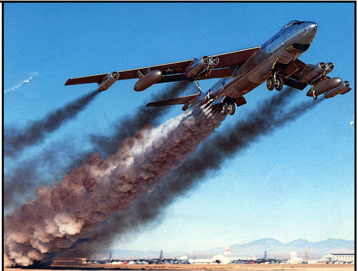
This B-47 has reduced its takeoff distance with the use of several "JATO" bottles attached to the rear underside of the airframe. . .
