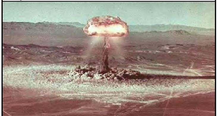
Buster "Charlie" ( 10-30-51 ) was a 14 Kt , test of a modified ( MK-4 ) bomb assembly with an experimental composite Uranium-Plutonium fission core assembly . . .
