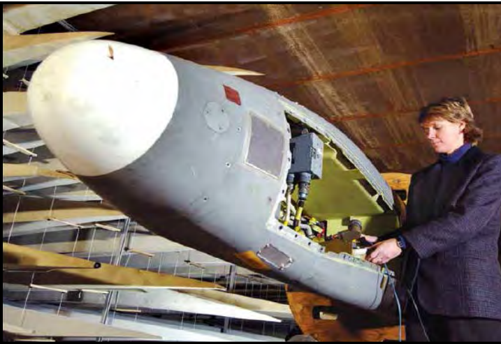
Michele Caldwell is shown here preparing a W-80 ( Sub-marine-Launched ) Cruise-Missile-3 for a variety of electro-magnetic anomaly ( interference ) tests. She says the new computer generated testing capabilities have allowed her group to take a comprehensive set of critical data which would not otherwise be possible. . . . .
