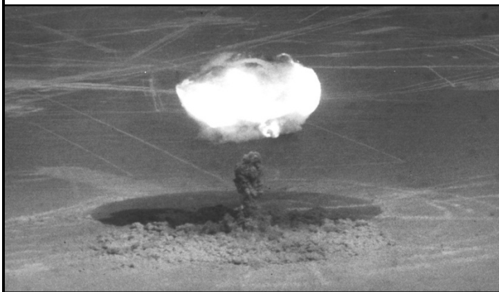
Ranger " Fox " was a 22 Kiloton "proof" test of a new Mk-6 composite fission core design. . .
