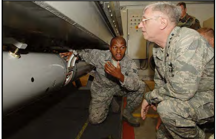
A visiting ( SAC ) General inspects a training version of a B-61 ( Hydrogen ) tactical nuke, in an underground Weapons Storage and Security System ( WS-3 ) vault at Volkel Air Base, The Netherlands. An access panel on the warhead is open, showing the interface for pre-flight set-up actions, including the PAL safety & arming station and the Dial-A-Yield ( DAY ) regulator device. . . .
