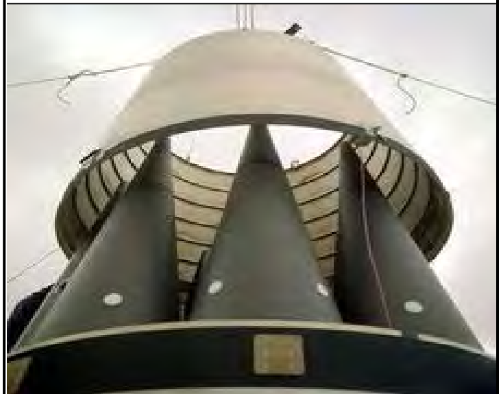
W-87 ( MIRV ) Warheads are assembled on top of a Minuteman-III Intercontinental Ballistic Missile ( ICBM ) . . . .
