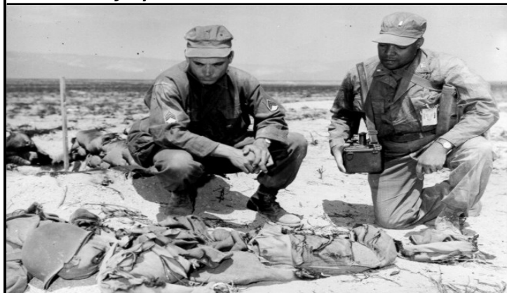
Military techs. are examining the remains of a "dummy" soldier destroyed by the "over-pressure" shock wave. . . .
