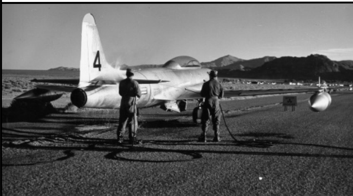
Now the "hot" airplane is washed down by the ground crew, who were not issued any radiation protective clothing or masks. . .
