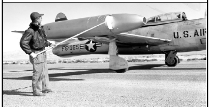
"Hot" ( cloud ) samples are removed from the wing-pods . . .
