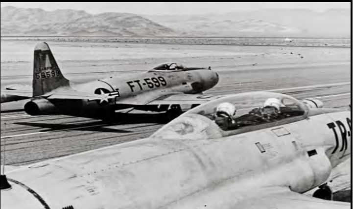
The QF-80 with the Chimp ( top ) is controlled by the QF-80 back-seat Officer ( bottom ) while lifting off from the "Indian Springs" runway, for a cloud sampling & radiation test mission . . .
