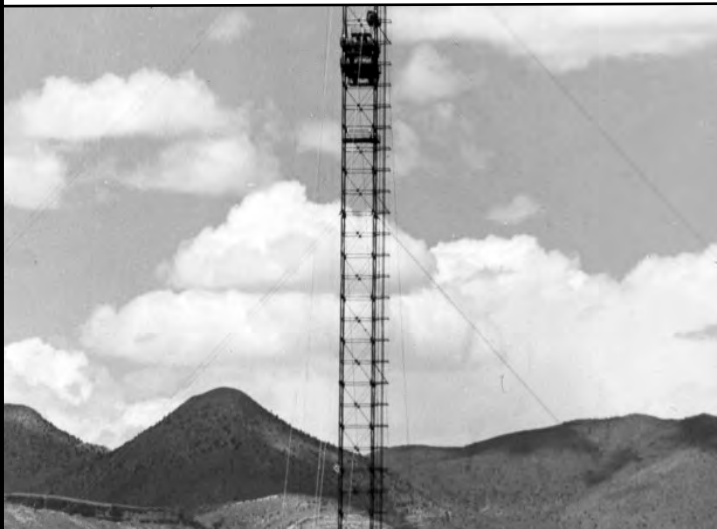
This is a typical NTS ( tower ) shot setup, showing the bomb device at the 100 ft. mark, as per the specs for this given test. . .
